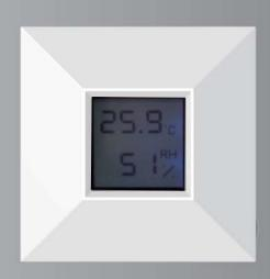
RS-23ZW is a wireless Z-Wave temperature and humidity sensor, offering a smart solution for healthier and comfortable home environment. Protect your home and belongings by monitoring the temperature and humidity levels in your home and receive immediate alerts if the climate fluctuates to unsafe or undesirable levels. Completely wireless, the RS-23ZW can be placed in any room of your home.
