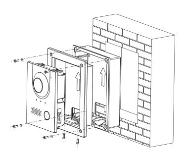
**Step1** Install the mounting box rear cover in the wall.
