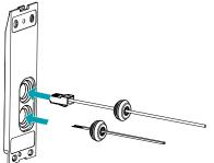
5 Connect the alarm terminal block to the alarm cable, and power terminal block to the power cable.
