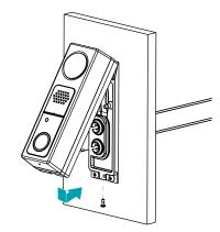
**10** Tighten the screw while pushing the bottom part of the camera body.
